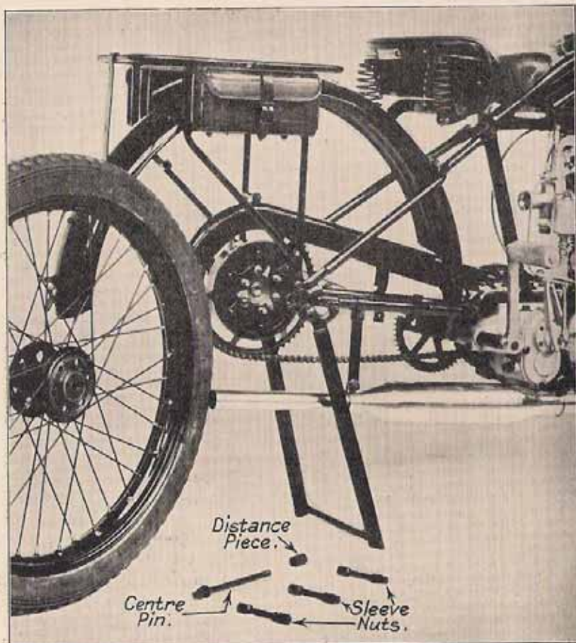
FIG. 50. THE REAR DETACHABLE WHEEL ON THE 3-49 H.P. MODEL The same system is adopted on all models with the exception of the H5
