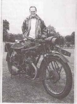
tubes to replace perished nubber and a magneto armature rewind - it is now out on the roads again, still bearing all the fittings and period accessories with which it was originally supplied. It even has the original chains and spark plug still in place and performing well. Only missing bits were the rear lamp and (strangely) one front mudguard stay, stolen while it was in store during the later war years.
