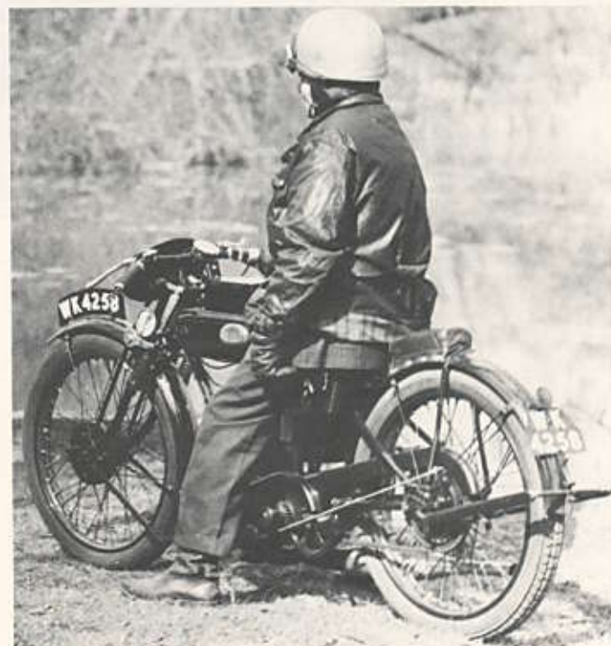
(Top) the upper tank rail is exposed by the flat tank. Small kneegrips and accessible toolbox. (Above, and preceding page) Tester Allen in a lakeside brown study
