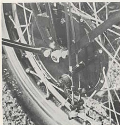
(Above) The inaccessibility criticised by Titch in his text. (Below) Coupled front brake can be over-riden by the hand lever
