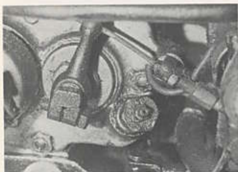
(Above) The inaccessibility criticised by Titch in his text. (Below) Coupled front brake can be over-riden by the hand lever
