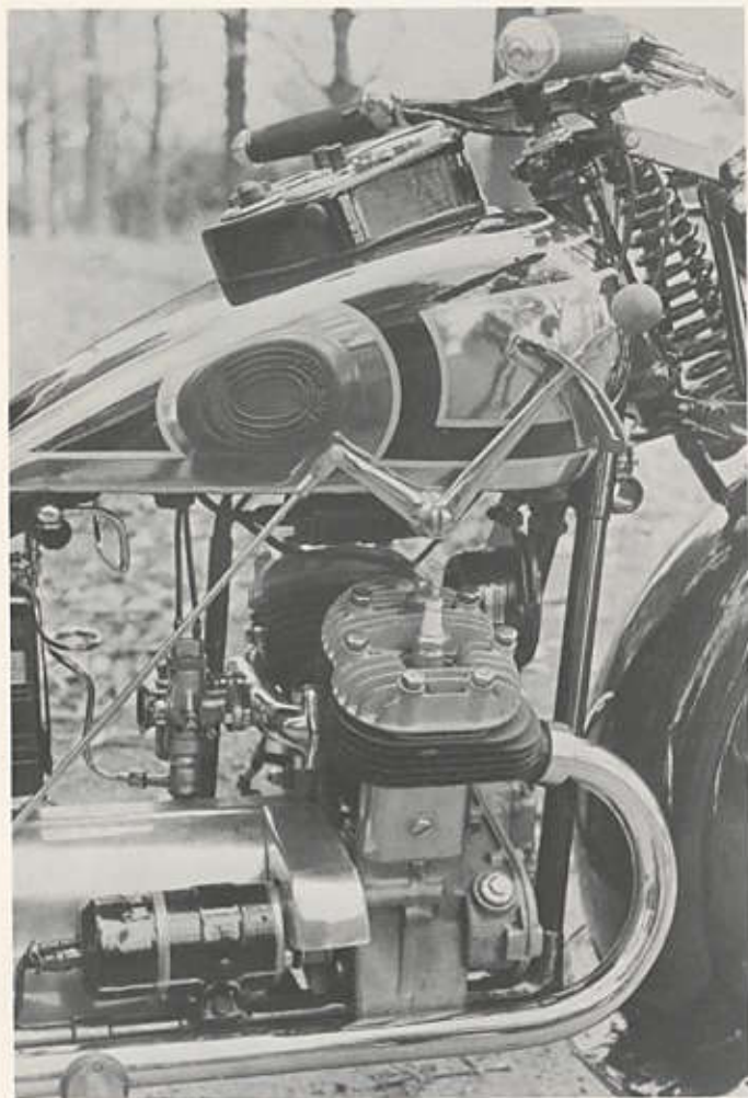
(Left) Twin camshafts to the sidevalves are chain driven at front of engine. (Above) A lengthy inlet manifold produces low-speed bias. (Below left) Generous steering lock so typical of the era and to be contrasted with modern superbikes. (Below right) Frame is of cradle type with duplex tubes. Sparks department by left footrest
