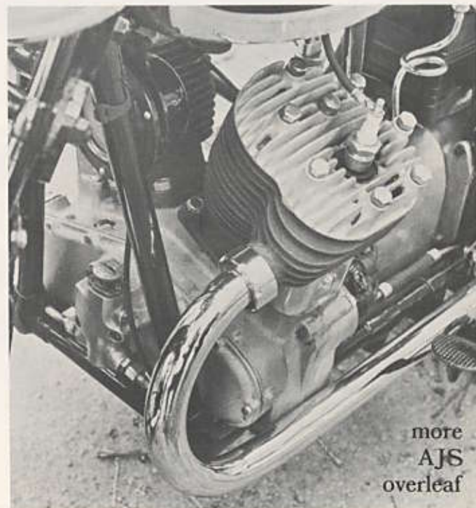
(Top) The non-adjustable abutments to the "clean" handlebars, so disliked by the tester. (Above) Smiths speedometer and Lucas electrical gear. The 3-gallon black and chrome tank is gold lined. (Below) Cylinder heads are light-alloy. The oil adjuster — see text for details — is seen at the front of the crankcase
