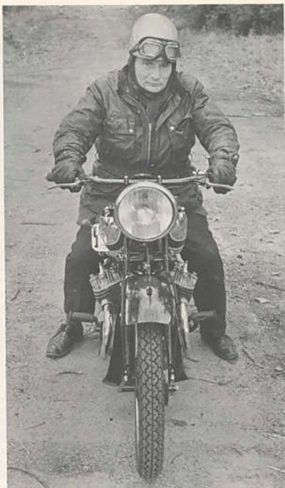
(Above) The minimal protrusion of the cylinder groups is clearly shown. They foul neither the knees, nor, as on a flat-twin, the feet. (Below) Allen eases the S3 into life. Full electrics and a centre stand are fitted. Dynamo is by right footrest. Handchange works on the up-for-bottom pattern. VE is a Cambridgeshire index mark used from 1928 on
