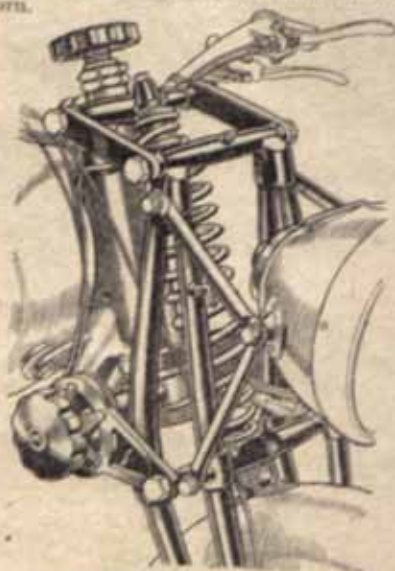
As a result of modifications the front forks fitted to machines in the "D" series now have a greater range of movement. Note the round-section tubing of which the fork girders are built, the heavier links and the rear-positioned shock-dampers
