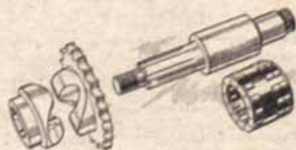
The mainshaft of the "D"-type engine has been increased in diameter and now runs in three rows of caged rollers, while splines for the shock-absorber are formed on the end of the shaft
