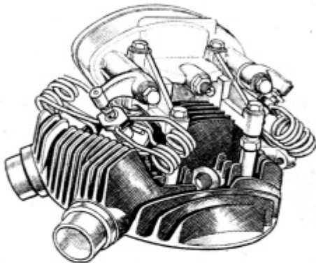
Arrangement of the overhead-valve rocker gear and hairpin valve springs on the 350 and 500 c.c. "Clubman" models
