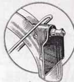
The rear number plate which has a shield bridging the gap between the plate itself and the mudguard.
