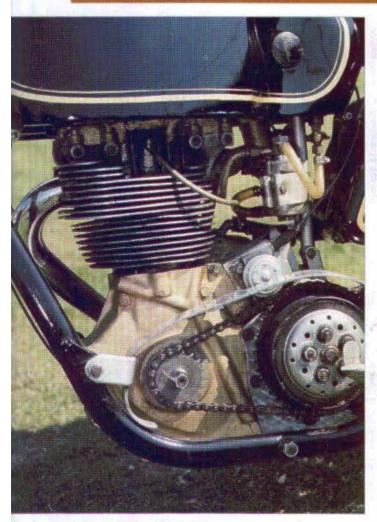
robably to help reduce development costs, the 7R engine followed the format more of traditional pre-war AJS race bikes with its single overhead camshaft single-cylinder engine and separate four-speed gearbox. Even so, the 7R was a completely new design, penned by Phil Walker.
