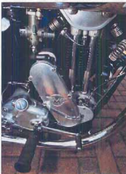
Dennis Kirk's 38/C80C has the later type gearbox, as fitted to the 1939 models.
