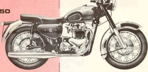
Engine, 745cc o.h.v. vertical twin (73mm bore x 89mm stroke): alloy cylinder head: parallel induction tracts with large diameter inlet valves: forged steel rockers: alloy pushrods: iron alloy tappets: single chain driven camshaft: built up forged steel crankshaft with large diameter central iron flywheel: plain big end bearings: two piece connecting rods: alloy pistons: (C.R. 7.6:1) cast iron cylinder: gear type oil pump: carburation by twin Amals: Lucas ignition with automatic advance and
