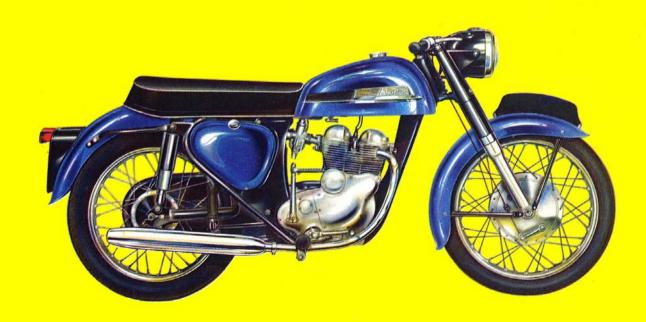
**SPECIFICATION.** As Jubillee except 63mm bore x 56mm stroke, and Roadholder forks and front Hubs colour scheme is blue and black.
