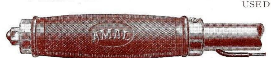
This illustration shows how NOT to bring the Cable into the bar as the cable is bent sharply too near to the Twist Grip and its free movement would be prevented.
