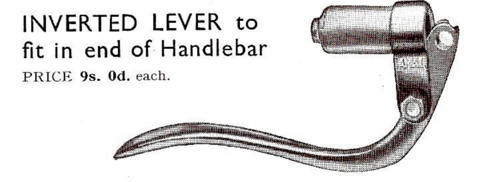
This lever is intended for fitting into the end of a 1" dia. handlebar of 14 gauge, the barrel bracket being '840" diameter. The pull is about \frac{3}{4}", but the fulcrum is longer than the above levers, so the purchase is less.
