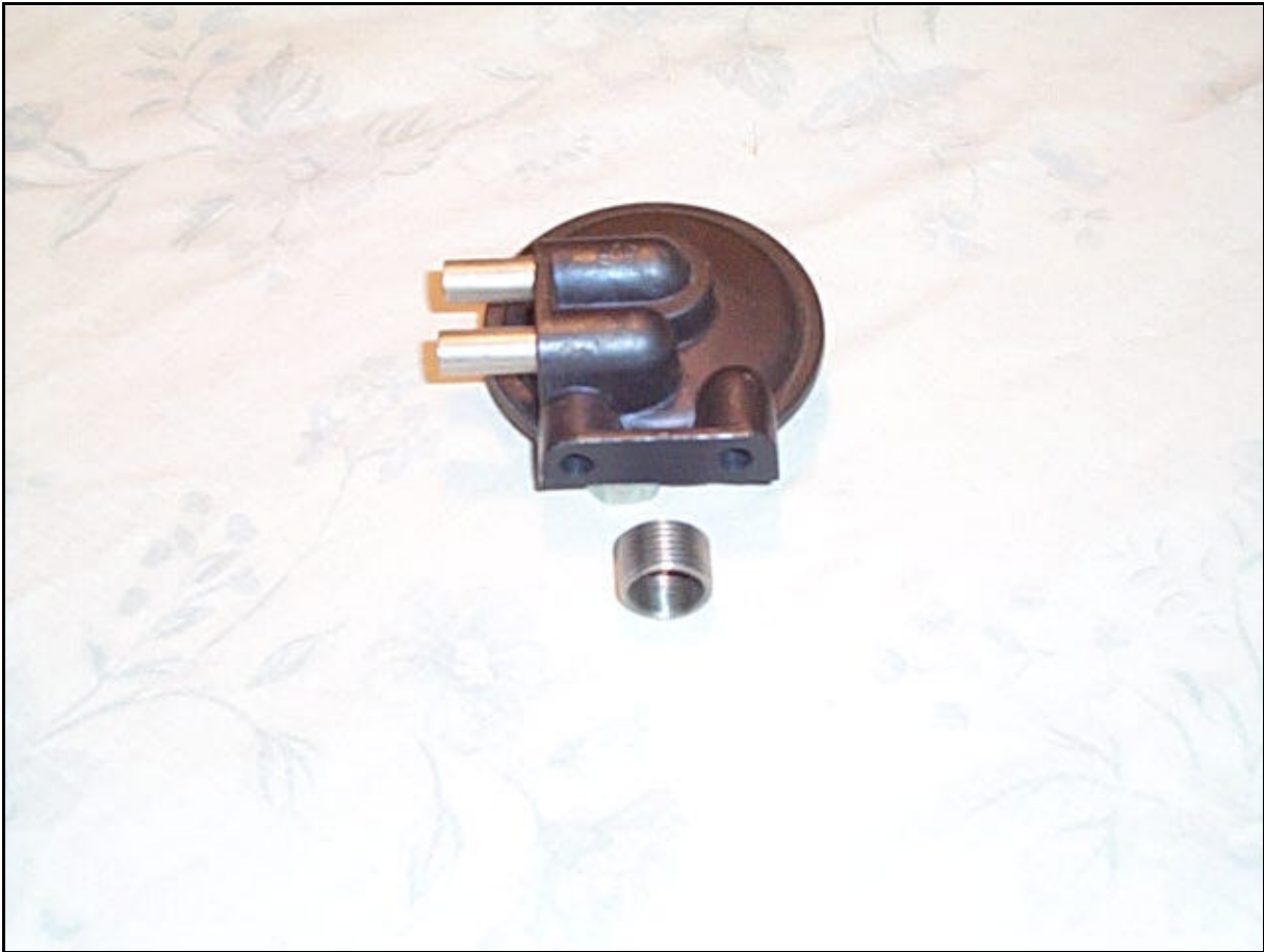
The Norton Commando after-market filter attachment and it's metric adapter.
