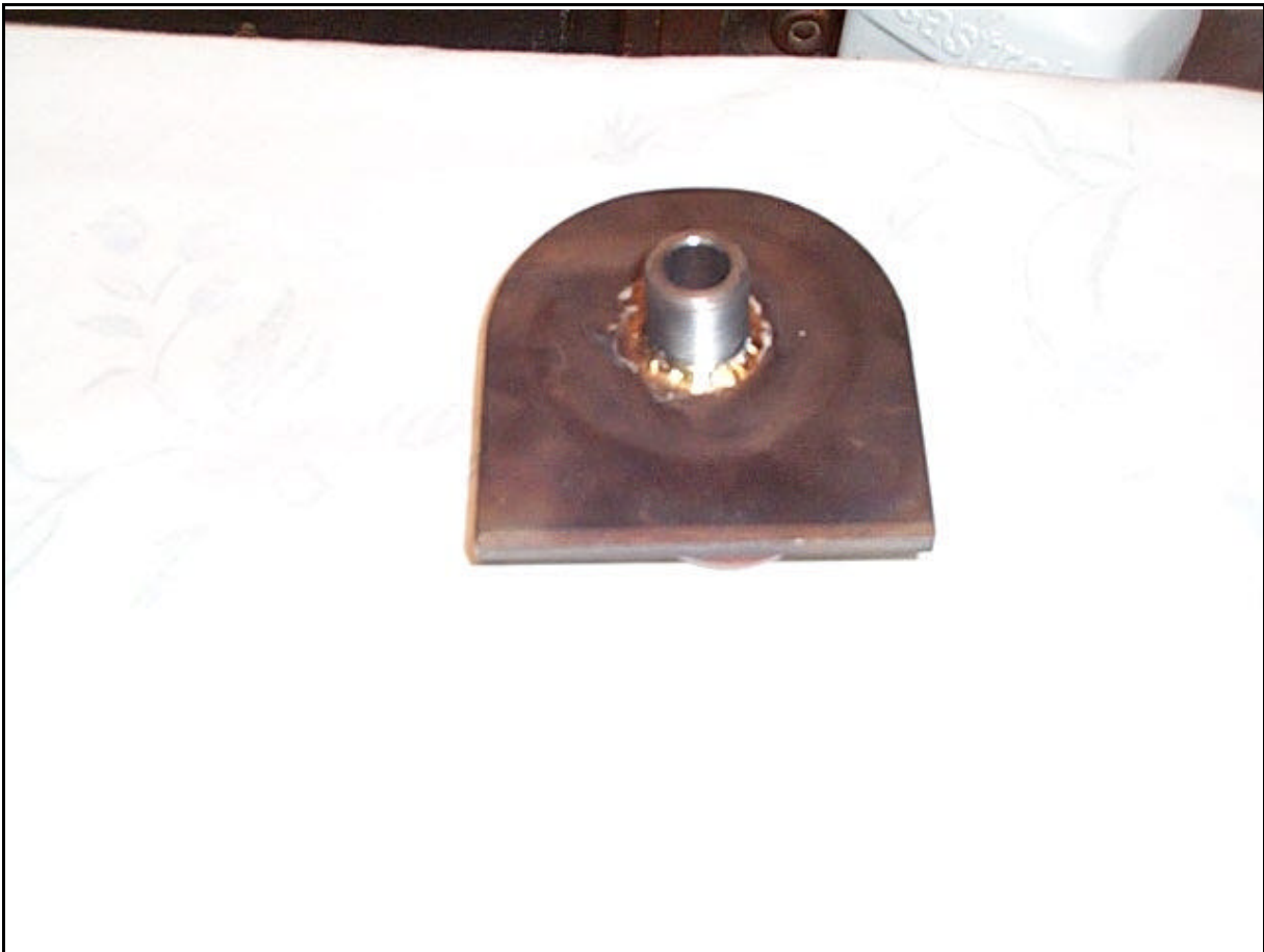
Metric pipe brazed in place.
