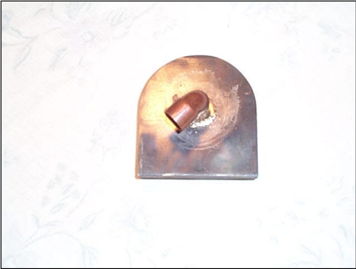
Filter plate with one fitting in place
