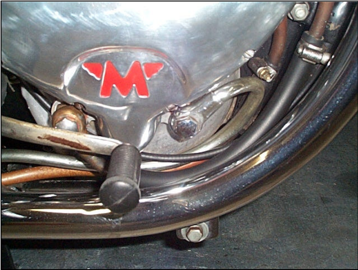
Correct connection of filter to return oil line
