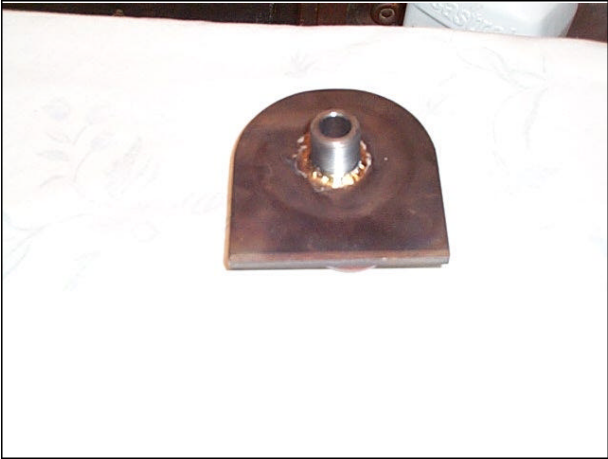
Metric pipe brazed in place.
