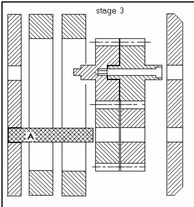
Stage 3: Assemble the pump and test it by hand, when it is running a bit tight look for high spots in the pump housing, or on the gears and remove them with a fine emery paper. It can also be the end play on the gears, I use 0,03 mm.
