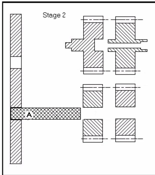
Stage 2: Make the axle (A) (steel or bronze) for the two free running gears, and give it a tight fit in the bottom plate of the pump.
