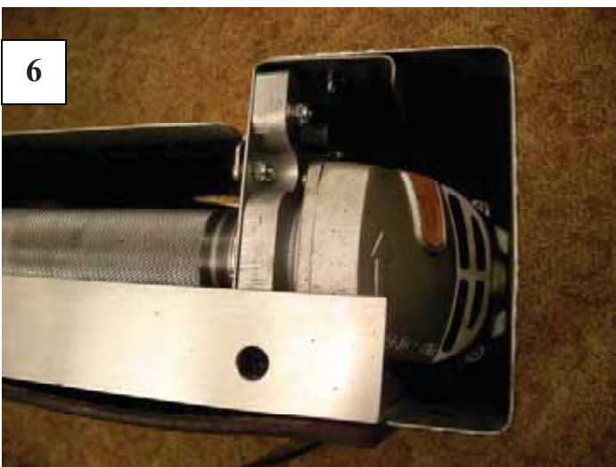
Figure #6 Shows the neatly located GMC 9" 1400w angle grinder power source.
