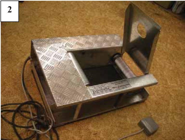
Figure #2 shows the hinged ramp to which the rear wheel is helped onto the rollers.
