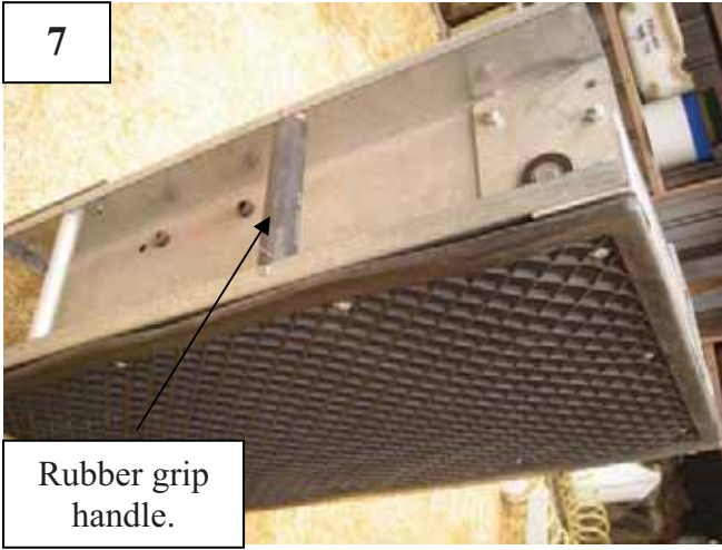
Figure #7 Clearly displays the rubber foundation mat and easy carry handle positioned for ease of balanced handling.
