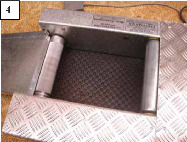
Figure #4 Indicating the gap in which the rear wheel is positioned. Unlike yours no side rollers are required.
