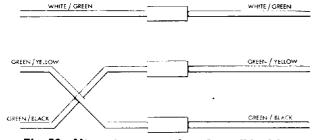
Fig. 56 Alternator connections for coil ignition motor cycles
