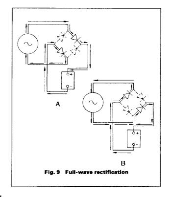
current is flowing in a clockwise direction; the righthand illustration (B) an anti-clockwise direction. With this arrangement the full output from the generator is utilised. That is, both the positive half waves and the negative half waves are used to charge the battery, shown by the graph C in Fig. 6, by inversion of the negative half wave.
