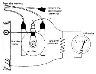
Fig. 68 Rectifier test in position
