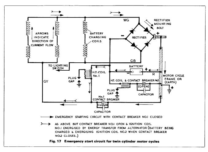
Another feature of the system is that the coil No. 2 eventually comes into operation during emergency starting, so that after a few seconds running on one cylinder, number two cylinder cuts-in and the engine functions as a normal twin-cylinder unit. It will not operate on both cylinders after a few more seconds because the rising battery voltage causes misfiring on the one cylinder.
