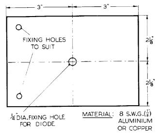
Fig. 52 Suitable heat sink dimensions
