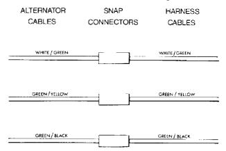
Fig. 57 Alternator connections for magneto ignition motor cycles
