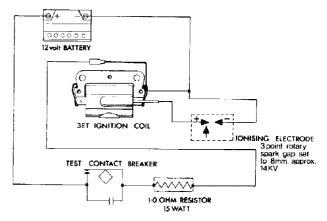
Fig. 74 Model 3 E.T. ignition coil bench test
