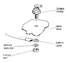
Fig. 38 Zener diode and heatsink
