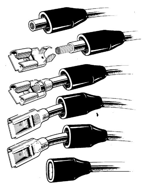
Fig. 63 Fitting instructions for Lucar connectors
