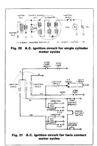
magnetic pulse in the alternator stator, which produces the energy pulse to feed the ignition coil primary winding, must be timed to occur at the firing point of the engine.
