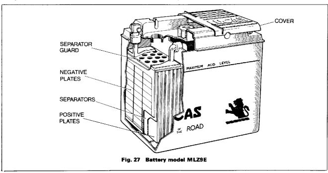
Occasionally, wipe away any dirt or moisture from the top of the battery, ensuring that the terminals are clean and tight. Never leave the battery in a discharged condition.
