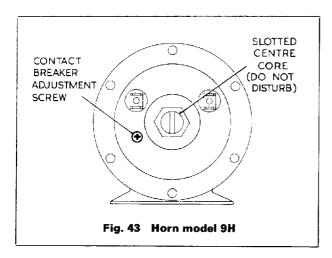
Operate the horn push and slowly turn the adjustment screw anti-clockwise until the horn just fails to sound. Release the horn push and turn the adjustment screw clockwise one notch at a time until the original performance is restored. This usually entails a clockwise motion of one quarter to
