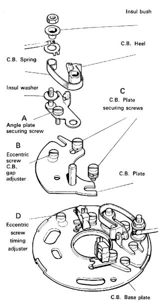
Fig. 28 Contact breaker model 6CA
