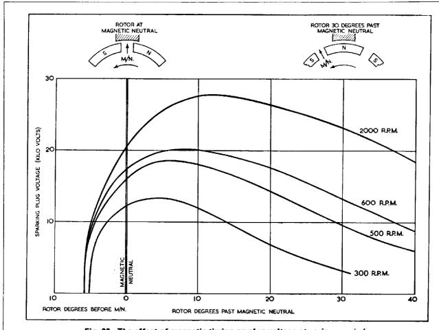
Fig. 22 The effect of magnetic timing on plug voltage at various rev/min
