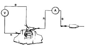
Fig. 70 Zener diode test
