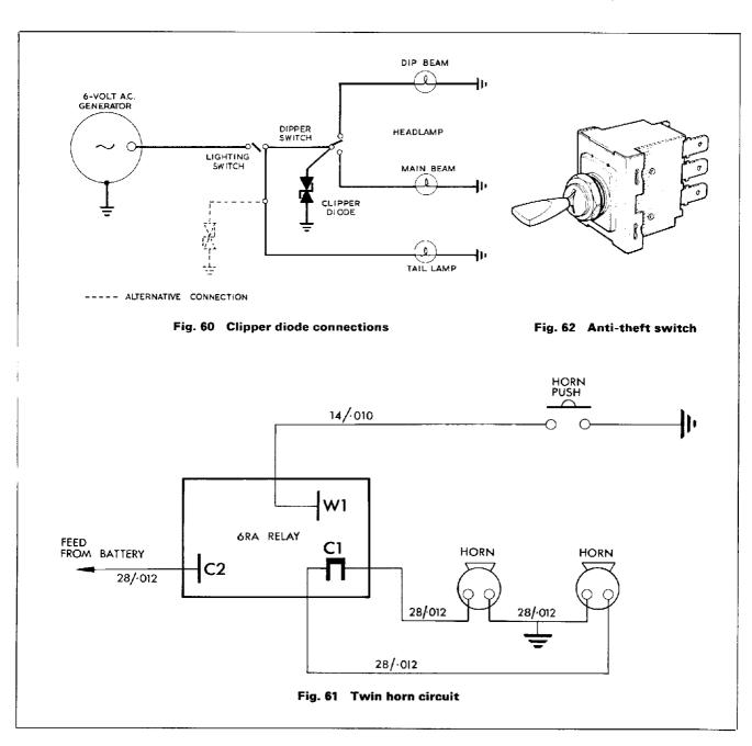
To fit the 45SA switch the connection between the positive (+) terminal of the battery and earth must be disconnected. The positive (+) terminal is connected to the No. 2 terminal of the 45SA switch, using 28/·012 cable. The No. 1 terminal is then connected to earth using the same type of cable. Disconnect the horn feed cable from the horn, and tape up. (If two cables are connected to the horn feed cable, these must be connected together before taping).
