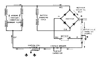
Fig. 16 Emergency start circuit for twin cylinder motor cycles with a distributor
