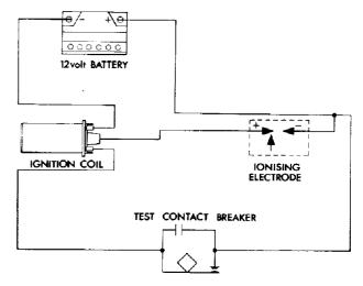
Fig. 75 Ignition coil bench test circuit
