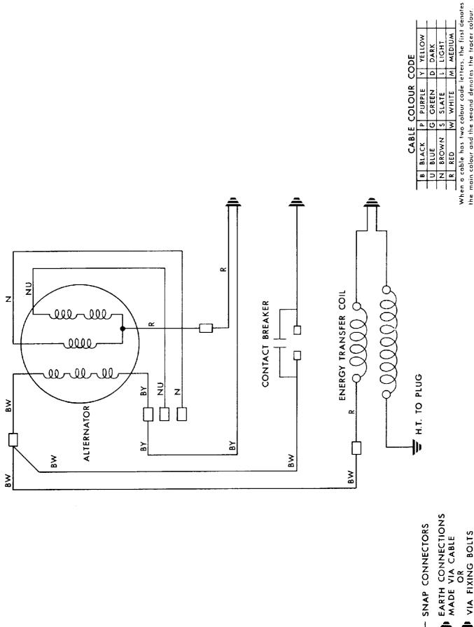
Fig. 80 Typical energy transfer for single cylinder machines (without lights)
