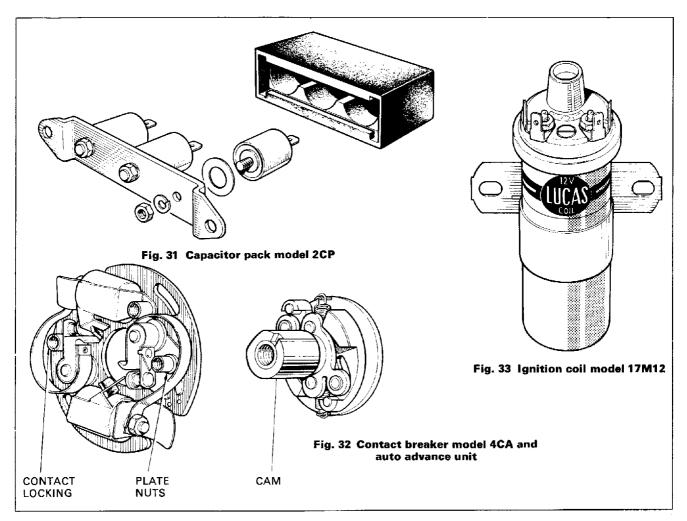
voltage could rise to 21,000 volts and normal insulation would break down especially in damp conditions. Ensure the chimney is clean and the H.T. connections are tight.
