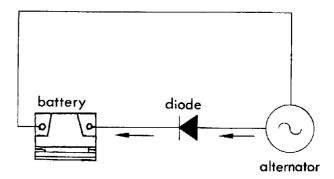
Fig. 8 Half-wave rectification
