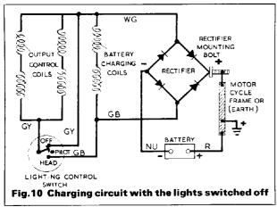
linked together and connected to a green/yellow cable. All the coils have the remaining terminals connected to a common white/green cable.
