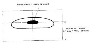
Fig. 41 Headlight adjustment
