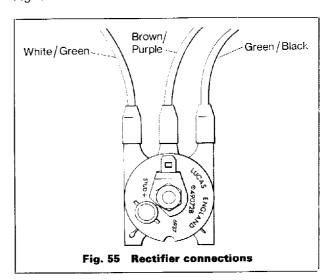
If the original circuit includes a White/Green (Green/White or Light Green) cable connecting a rectifier terminal to the lighting switch, this must be disconnected at the switch and taped up.
