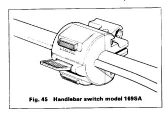
The left-hand switch controls headlight dipping on the lever, headlamp flash on the upper push button, and horn on the lower push button. The right-hand switch controls the direction indicators on the lever, the starter solenoid on the upper push button, and the ignition cut-out (or kill) on the lower push button.
