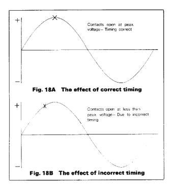
will not open at the peak of the voltage curve, see Fig. 18 (B) and consequently the spark will be weak. REMEMBER, IGNITION TIMING IS CRITICAL.
