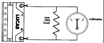
Fig. 65 High rate discharge test
