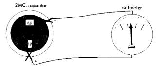
Fig. 73 Capacitor bench test
