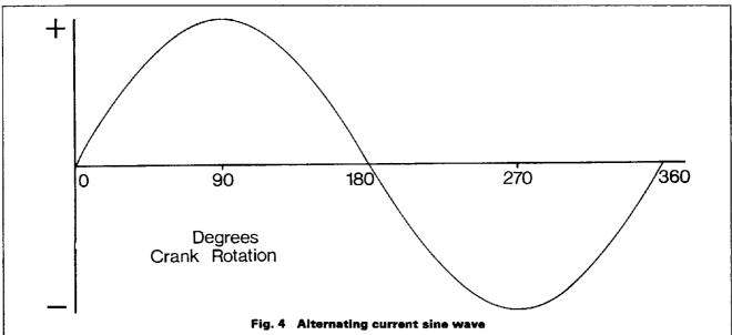
negative direction reaching a maximum at 270°, then gradually reduced again, becoming zero at 360°. This cycle is repeated as long as the magnet is rotated.
