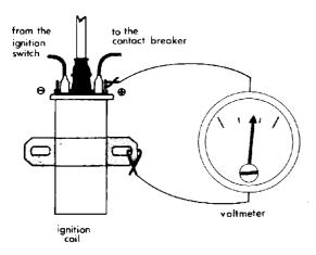
Fig. 71 Coil and contact breaker circuit test
