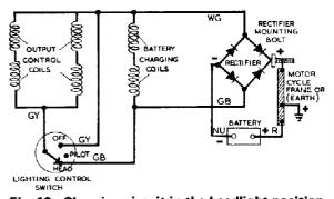
Fig. 12 Charging circuit in the headlight position
