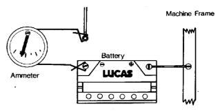
Fig. 66 Maximum charge rate test
