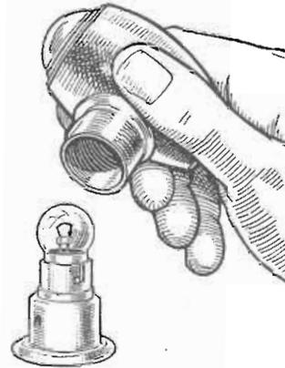
To gain access to the bulb withdraw the securing screw on the lamp stem and then pull the body away from the base. The bulb can then be removed from its holder. Replace the lamp body and secure with the screw.
