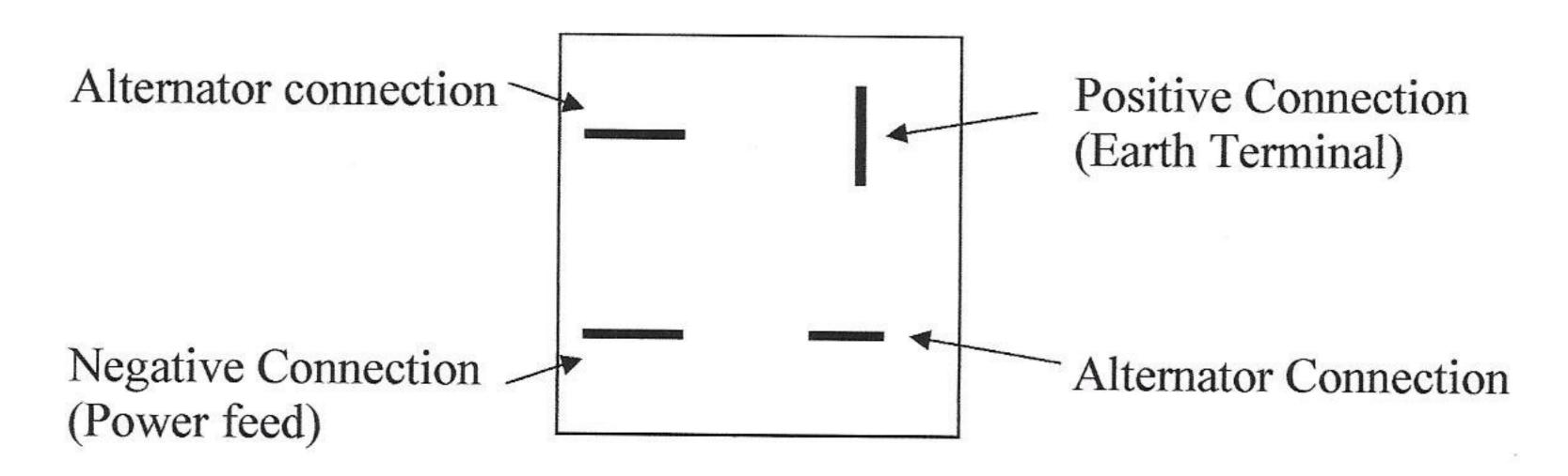
This rectifier will replace the plate one normally fitted. The connections shown are correct for bikes with positive earth, standard Lucas motorcycle alternator.
