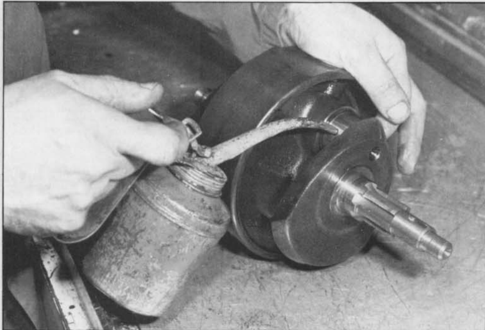
Force oil through the crank feed holes to check flow before assembly.
