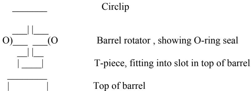
With the unit off, note that there are two oil holes, with O-rings. Nothing much can be seen through the lower one, but in the upper one part of the rotating barrel is visible. Note the vertical channel, 3mm wide, that ends just below the top of the hole when the adjuster is at position 1.
