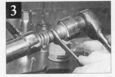
spanner) (pic two). Push the slider up until internal spring and damper rods are exposed.
