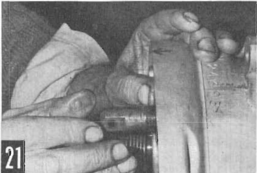
21 Do up mainshaft nut, replace clutch operating body and screw lock-ring in finger tight. Line up body with pencil mark on case and tighten ring
