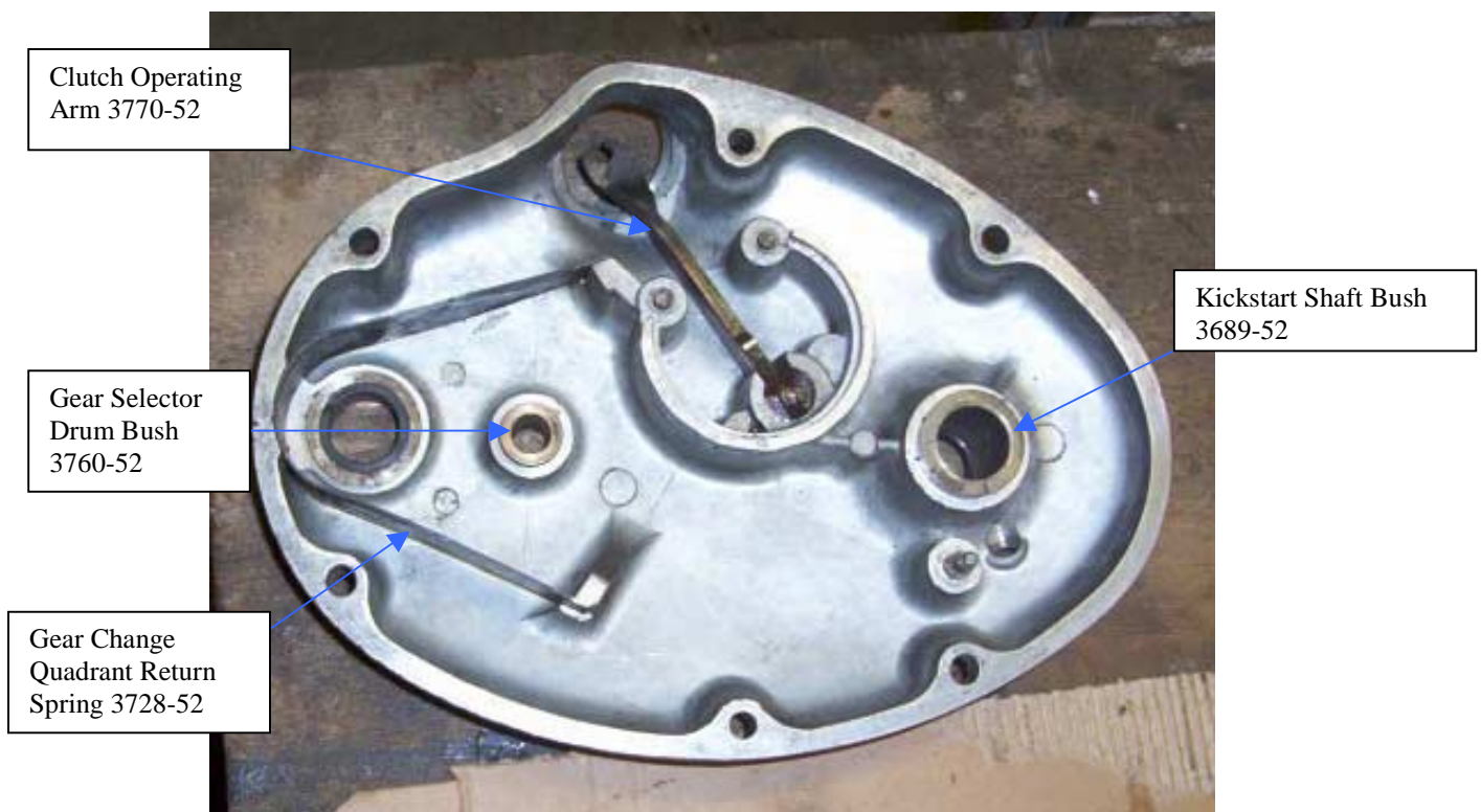
View on Inside of Kickstart Case
