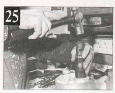
B ACK in Bill's workshop for the rebuild all parts were cleaned in paraffin and the gearbox shell warmed up to ensure the output shaft bearing dropped in easily. The seal and its sleeve (pic 24) were first tapped into place (pic 25) and the bearing, which had been cooled in the freezer, dropped in from the inside (pic 26) and was tapped home. When driving bearings home it is important to make sure the case is solidly supported, otherwise the force could cause it to crack.
