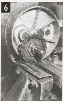
clutch operating arm mechanism was undone with a 'C' spanner. Bill used a screwdriver to make up for his spanner being too big but stressed it was not really the right way to do things. Maybe not, but it worked (pic 8). The alternative is to use a hammer and a punch, but that can easily damage the mechanism.
