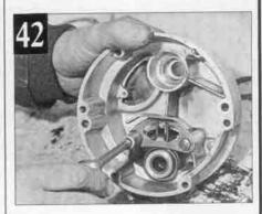
• As the original wasn't in bad condition Bill decided it would be alright to risk it and slotted the unit into place (pics 41, 42 and 43). With the gasket fitted and shafts oiled the outer cover then slipped into place; movement on the gearchange and kickstart mechanisms checked; and the cover screws refitted.
