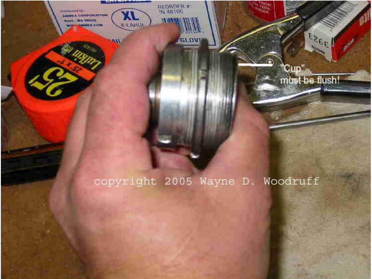
Fig 7: Side view of Fig 6 - showing cup MUST BE FLUSH with housing!
