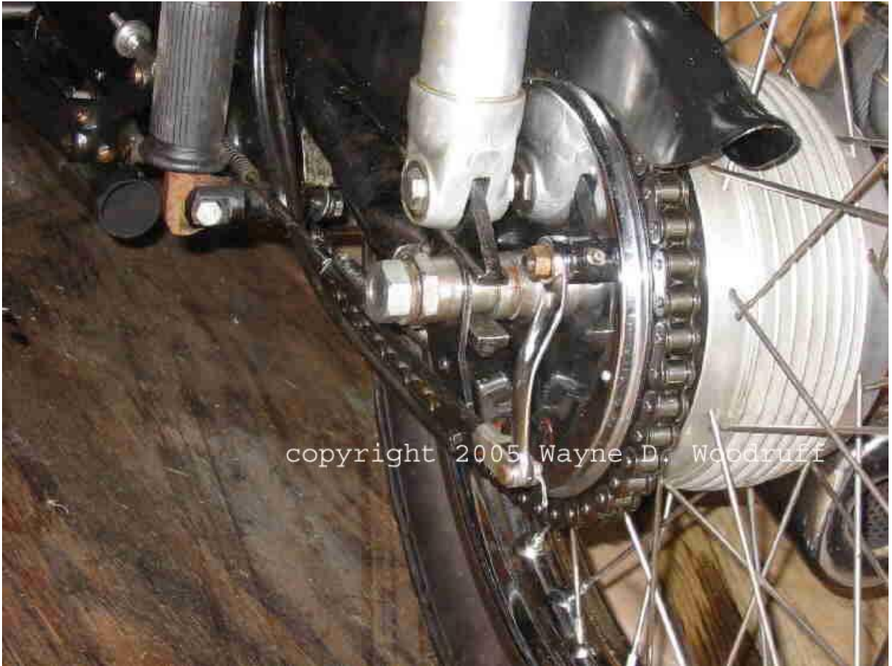
Fig 14: Left side of rear wheel showing all installed components
