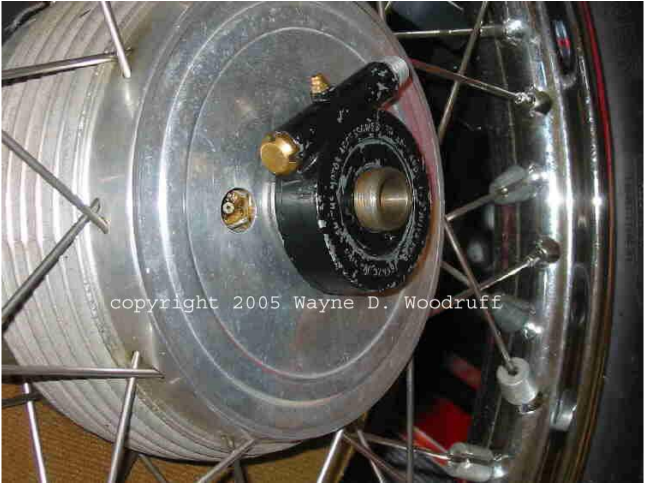
Fig 10: Speedo drive installed
