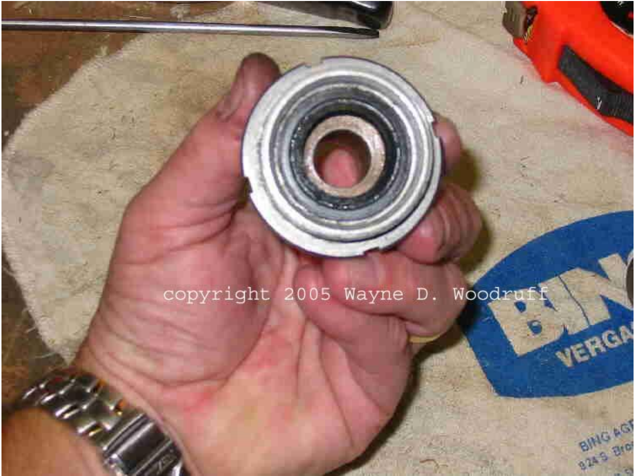
Fig 5: Rubber (or felt) seal now in place. You must work this to fit within the opening in the housing.
