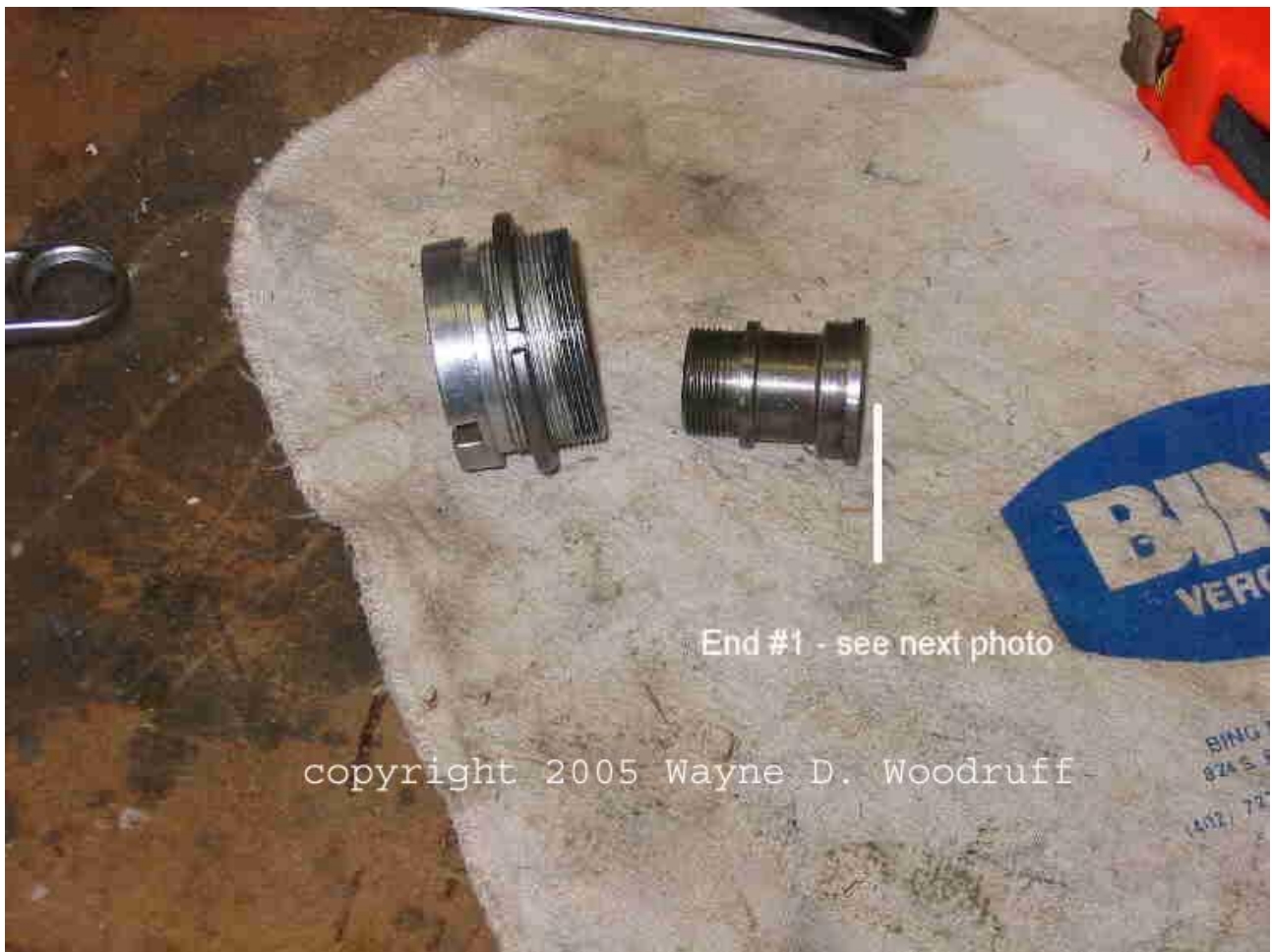
Fig 2: The threaded axle the the speedo drive attaches to as about to be inserted in the retaining ring
