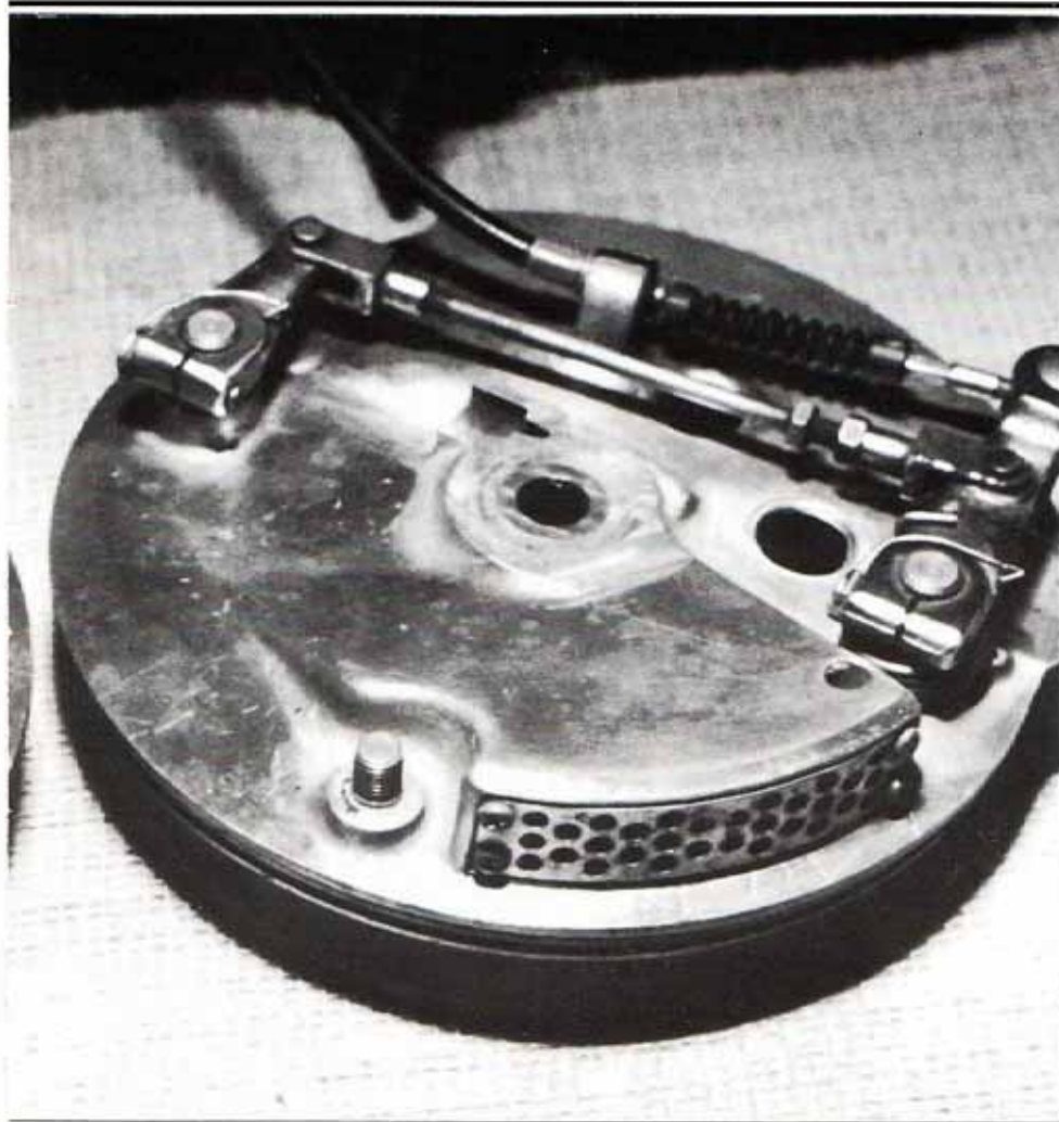
Left and right: Suzuki four shoe brake backing plates after machining.
