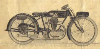
3.19 h.p. 3-SPEED A.J.S. OVERHEAD VALVE RACING MACHINE
