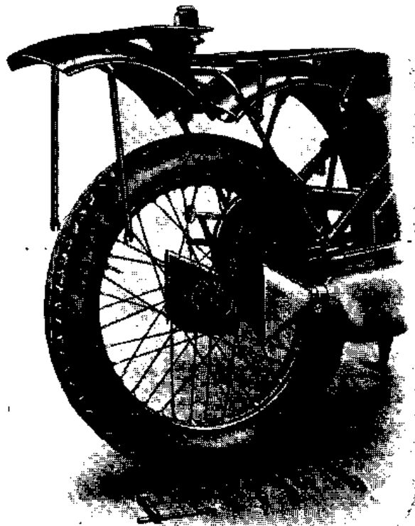
Illustration 12. THE A.J.S. QUICK DETACHABLE WHEEL.
