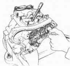
Removing the camshaft sprocket nut
