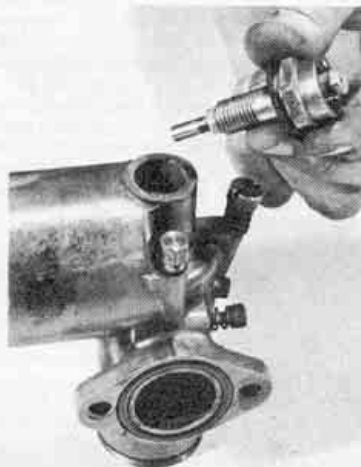
Removing the jet holder and jets
