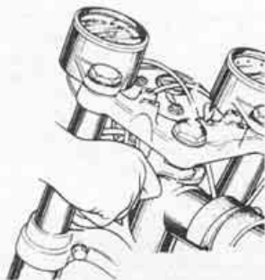
Adjusting the steering head bearings (pre-1971 models).
