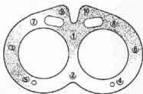
Cylinder head tightening sequence
