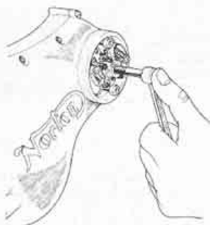
Removing the advance mechanism
