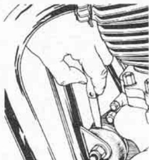
Checking clearance in the front engine mounting (1974 and earlier)
