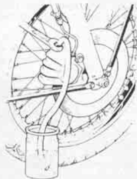
Bleeding the front disc brake
