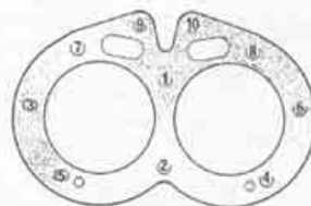
Cylinder head tightening sequence; reverse the order when removing the head
