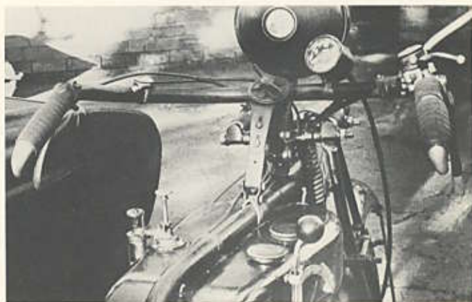
(Left) In typical vintage AJS manner the cylinder heads can be detached in a trice, complete with valves. (Above) The chair wheel interchanges with either on motorcycle. (Below) Brampton forks have fore and aft snubber springs
