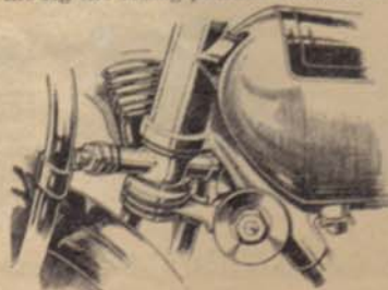
The massive head, showing the steering-lock stop incorporated with the damper attachment.
