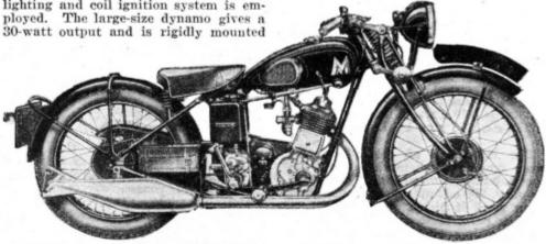
The new 250 c.c. s.v. Matchless is similar to the "Sports 250" except for the engine and silencer. Coil ignition with large dynamo and battery, are standard on both models.
