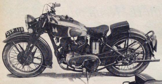
(Left) The prop-stand in action. The standard equipment includes an air cleaner, voltagecontrol unit and a four-gallon petrol tank
