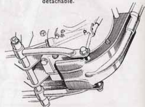
This crankcase shield is a standard A.J.S. fitting. It forms a splendid protector and is anything but unsightly.
