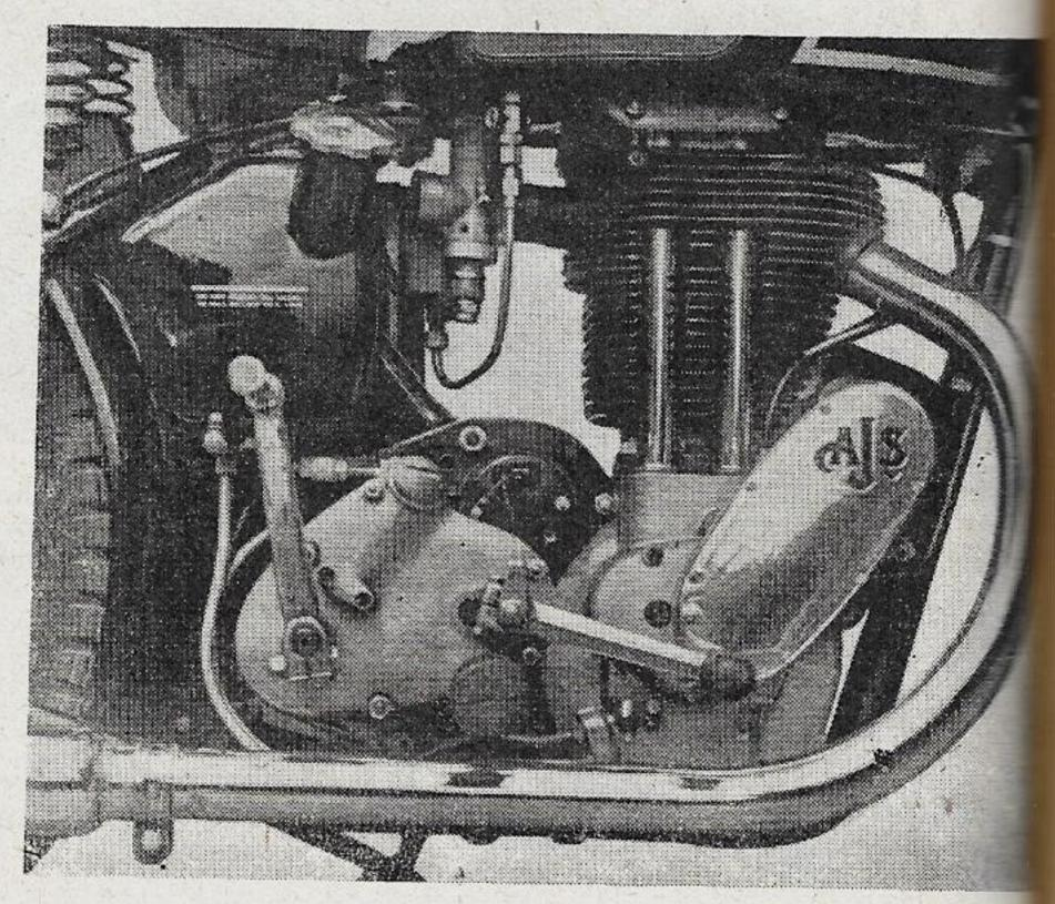
ing is provided for chain adjustment. The automatic voltage control unit is mounted beneath the saddle. The offset Amal carburetter is insulated from engine heat by a thick Bakelite distance piece.
