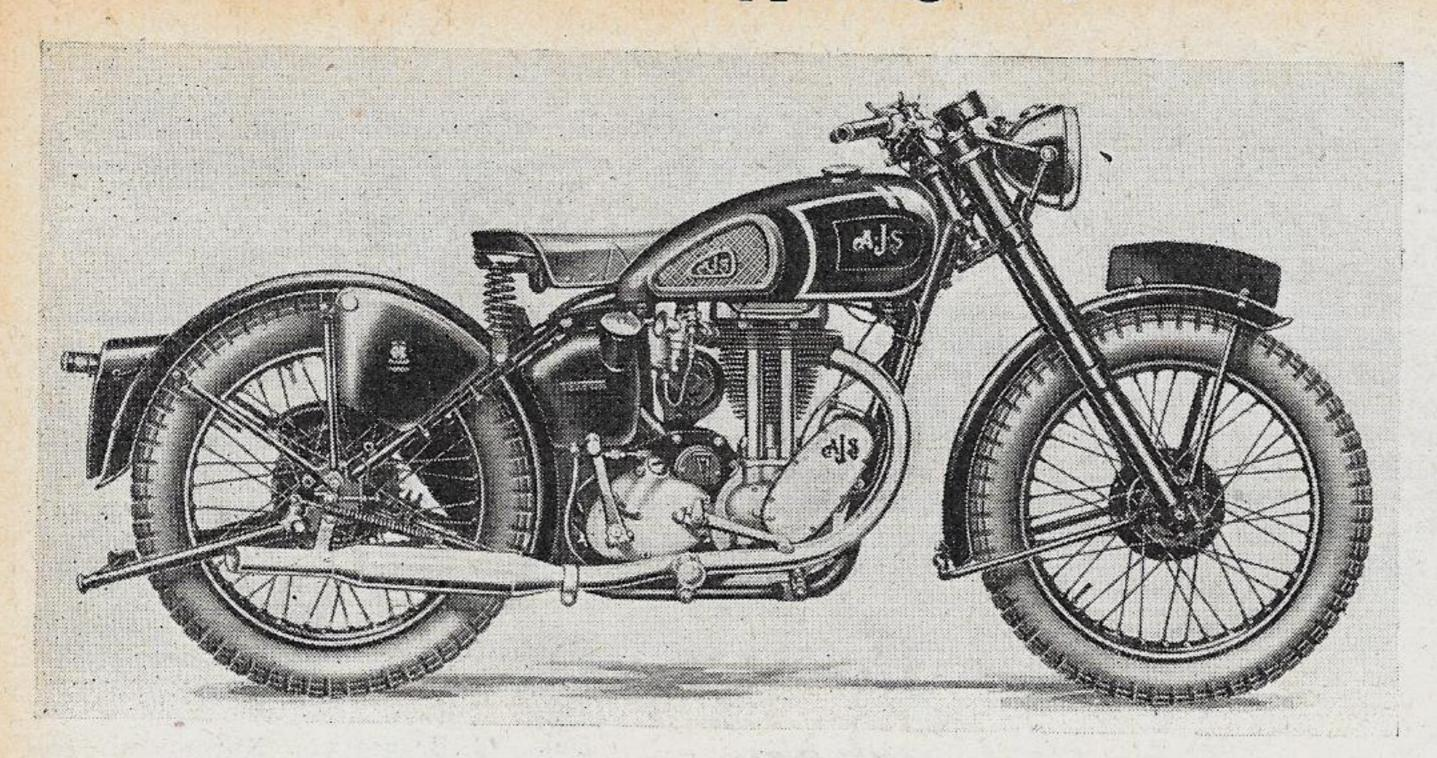
Off-side view of the new "350" Model 16 M. The "500" Model 18 is identical in appearance save only for deeper cylinder fins and an exhaust pipe which passes below the footrest.
