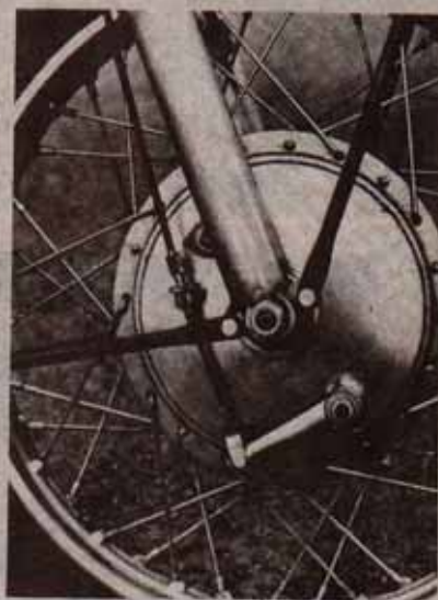
Removing the screw at the bottom of the forks allows the owner to change weight of the suspension oil. Single leading shoe brake works well.
