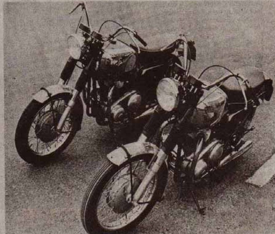
Both look the same but one is a year old. The newer machine, on the left, has a key ignition and the new Amal Concentric carburetors.
