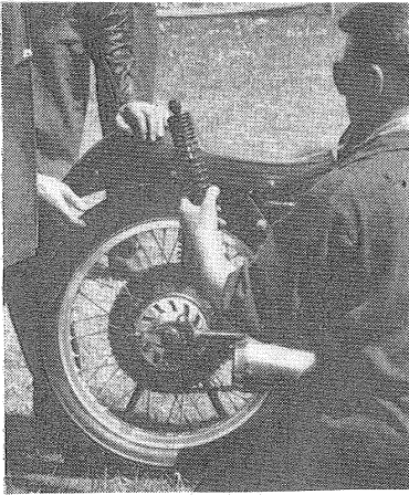
Changing the rear-suspension units of a 7R. For several years riders complained in vain about the uncertain damping provided by the original units; eventually they were replaced by Girling equipment
