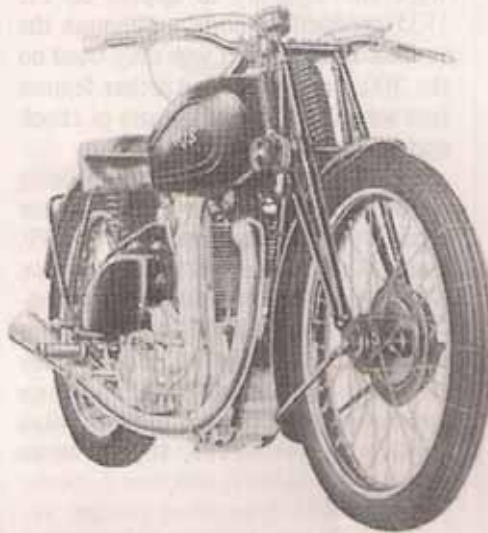
From the maker's 1938 advance catalogue - well, leaflet really - this is the racing Model 7R. The 500s and all road-going versions were dropped from this season. The remote float mounting isn't shown, although it was introduced in this year
