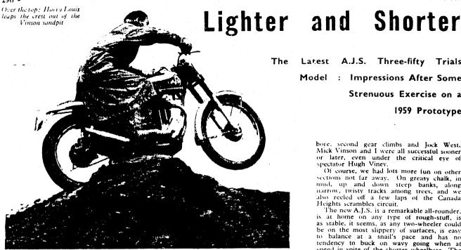
PRODUCTION trials models have changed quite a bit during the last decade. In the late 1940s they had solid frames and engines that pulled unfalteringly at tick-over speeds, but were not particularly sprightly on a wide throttle. The weight saving was limited to using narrow-blade mudguards and smallish fuel tanks, and removing lighting equipment. Riding styles were different, too; the top boys were, above all, balancing artists.
