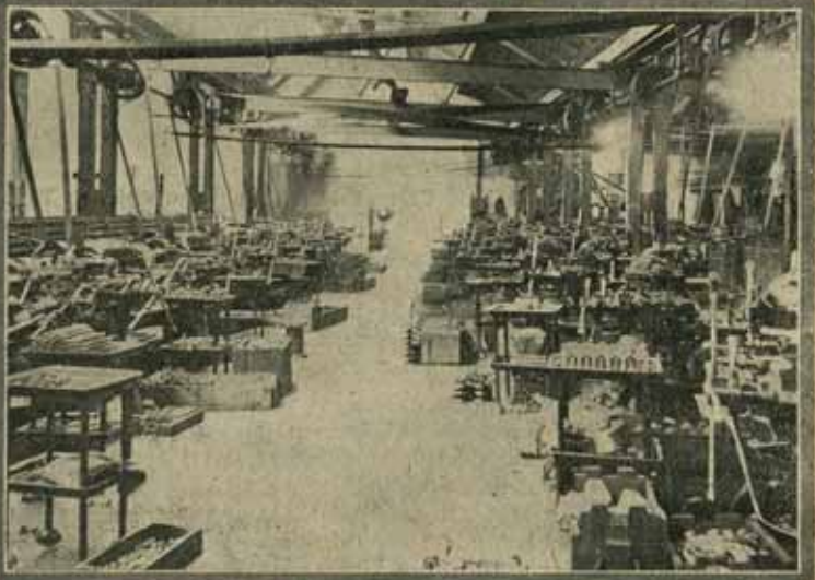
The capstan department is equipped with No. 4 Herbert capstans.
