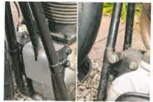
FAR LEFT Toolbox on both 350 and 500 is a simple pressed metal affair.
