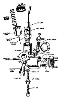
The new Manobloc carburetor features a float bewl and mixing chamber cast as one unit. A hinged float and nylon float needle are used.
