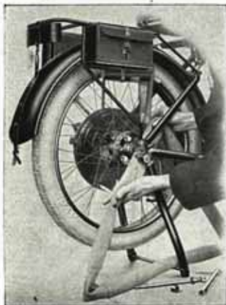
A.J.S. DETACHABLE WHEEL Centre-Pin of Rear wheel withdrawn to allow Inner Tube to be completely taken out and replaced without detaching the wheel!
