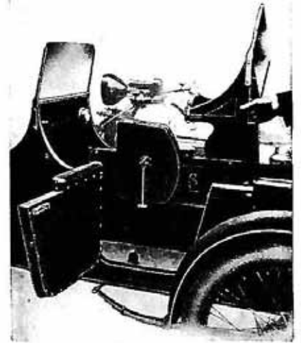
Showing Seat folded back and the dash raised.
