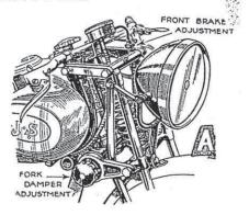
A well-known feature of "A.J.S." Motor Cycles is the exceptionally sturdy front fork assembly shown above. Note the accessible finger adjustment for the front brake, the convenient shock absorber adjusting knob, and the stiff headlamp mounting.
