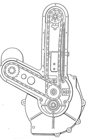
The illustration above shows the well-known "A.J.S." Camshaft Chain drive in which is incorporated a tensioning device and re-action damper. This method of driving the camshaft was employed in our actual T.T. Models, and it will be remembered that "A.J.S." was the only make to obtain 100 per cent. finishers in the Senior Race, each entrant gaining a Replica.
