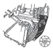
This illustration shows the Vernier Setting Device used on Models 35/5, 35/6, 35/8, 35/18 and 35/9 which allows for quick and accurate ignition timing.
