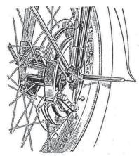
This cutaway view of the highly efficient front brake used on all Models except 35/12, 35/5, 35/16 and 35/4, shows the alloy drum with its cooling fins, which serve also to stiffen the drum to prevent discortion, the aluminium alloy brake shoes, and the neat manner in which the operating cable is concealed by passing through the front fork tube, whence it emerges at the finger adjuster shown in the top illustration.
