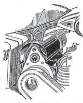
On the Big Twin Models the magdyno is protected by the efficient shield shown above, which ensures reliable Ignition even in tropical downpours.
