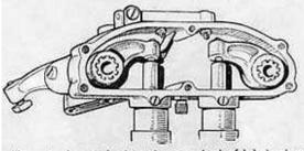
Above is shown the ingenious method of lubricating the ball-ends of the push-rods on the "Sports 500" machine. Tiny jets fed with oil from the main pump squirt oil just where it is needed to ensure silent operation and freedom from wear.
