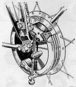
Above is shown the brake used on the "Sports 500" and some other models. The brake drum is made of centrifugally-cast chromidium-iron alloy and is stiffened by deep fins which also serve to ensure adequate cooling.
