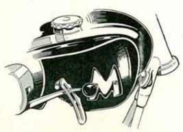
All "Matchless" petrol tanks are distinguished by the embossed chromium "M" which is carried on each side of the tank at the front end. The tank is finished in hard stoved glossy black enamel with gold lines, and a very handsome appearance is given by the contrast between the black enamel and the chromium "M." Note also the way in which the tank is mounted on rubber buffers to absorb vibration.
