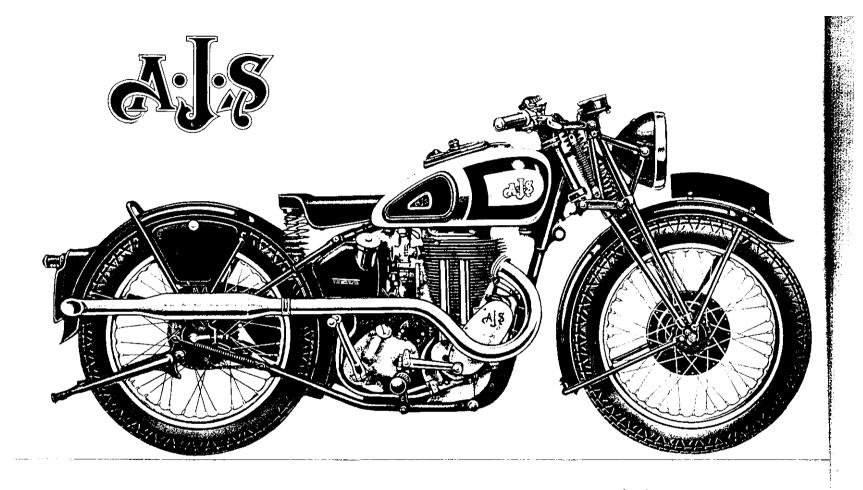
498 c.c. O.H.V. De Luxe Model. Single-port exhaust system. Petrol tank chromium plated with black panels lined silver and blue. Wheel rims chromium plated with silver centres and black lines. Sports mudguards. Check-spring front forks. (For full specification see pages 4 and 5.)
