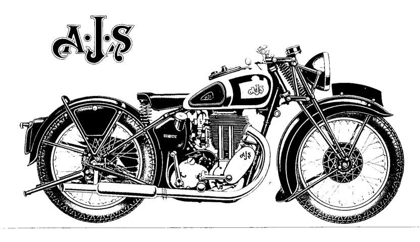
498 c.c. O.H.V. De Luxe Model. Two-port exhaust system. Petrol tank chromium plated with black panels lined silver and blue. Wheel rims chromium plated with silver centres and black lines. Valanced mudguards. (For full specification see pages 4 and 5.)
