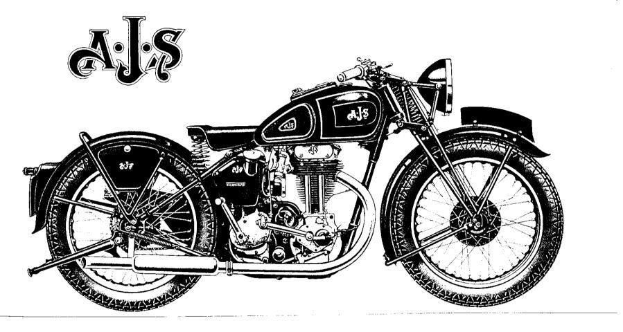
246 c.c. O.H.V. Standard Model. Coil ignition, single-port exhaust system. Petrol tank finished in black and gold. (For full specification see pages 4 and 5.)
