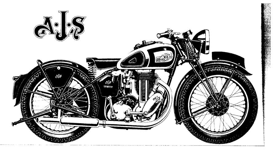
347 c.c. O.H.V. De Luxe Model. Magneto ignition, two-port exhaust system. Petrol tank chromium plated with black panels lined silver and blue. Wheel rims chromium plated with silver centres and black lines. (For full specification see pages 4 and 5.)
