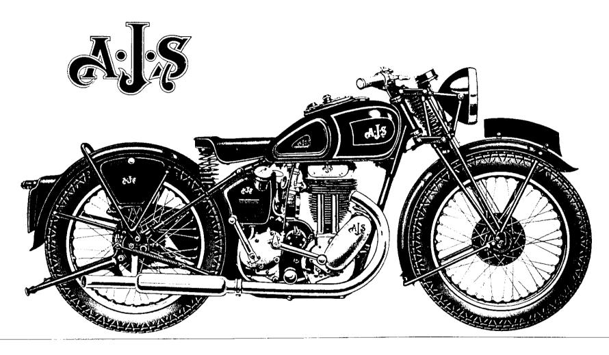
246 c.c. O.H.V. Standard Model. Magneto ignition, single-port exhaust
