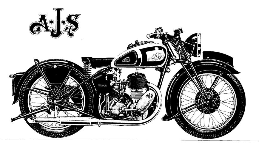
498 c.c. Side Valve De Luxe Model. Petrol tank chromium plated with black panels lined silver and blue. Wheel rims chromium plated with silver centres and black lines. Valanced mudguards. (For full specification see pages 4 and 5.)
