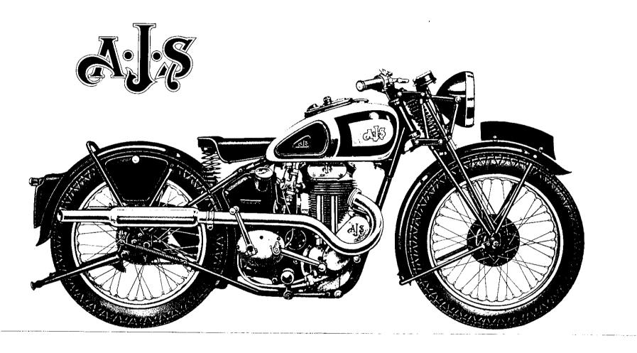
246 c.c. O.H.V. De Luxe Model. Magneto ignition, two-port exhaust system. Petrol tank chromium plated with black panels lined silver and blue. Wheel rims chromium plated with silver centres and black lines. (For full specification see pages 4 and 5.)
