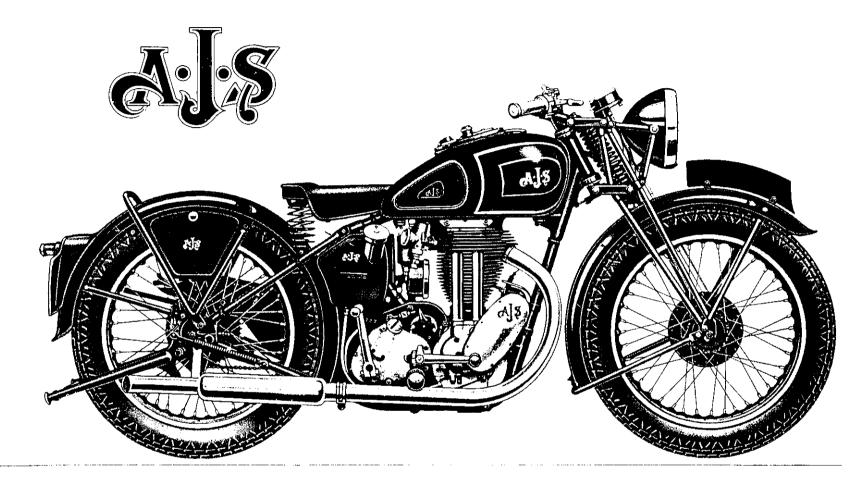
$347~\rm c.c.$  O.H.V. Standard Model. Magneto ignition, single-port exhaust system. Petrol tank finished in black and gold. (For full specification see pages 4 and 5.)
