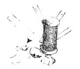
On all the "De Luxe " series and "Silver Streak " models. the speedometer is carried on the neat bracket shown in the illustration, the position being such that the rider can see the dial without removing his vision from the road ahead.
