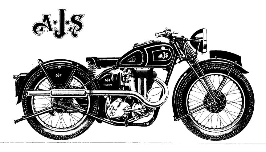
347 c.c. O.H.V. Standard Model. Coil ignition, single-port exhaust system. Petrol tank finished in black and gold. (For full specification see pages 4 and 5.)
