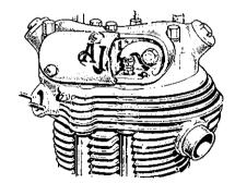
The illustration on the left shows the latest type of A.J.S. overhead valve gear, with the rocker box detached from the cylinder head to show the disposition of the valve springs and the push rods which operate the overhead valve rockers
