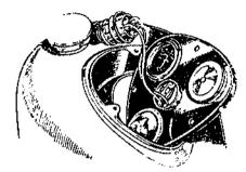
The instrument panel can be passed through the tank without disturbing the wiring.
