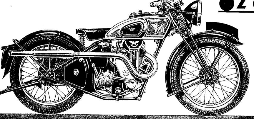
246 C.C. OJHLV, TWO PORTS MAGNETOSIGNITION FOR PULL SPECIFICATION SEE PAGES 25 and 8
