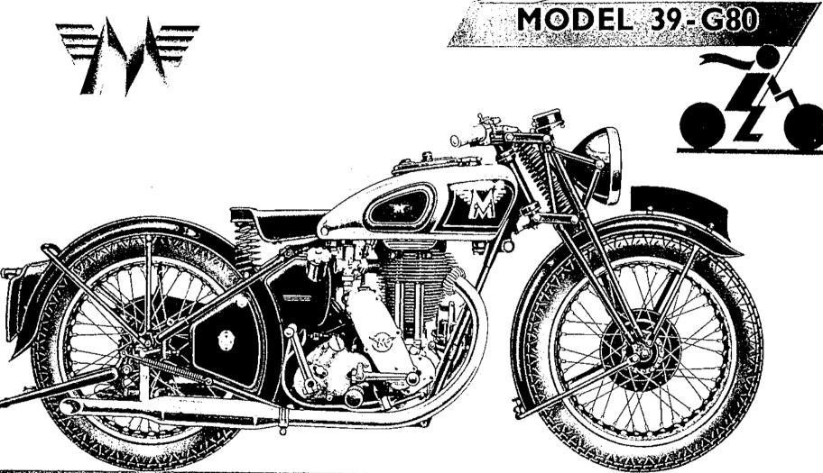
498.C.C. O.H.V. TWO PORT; MAGNETO IGNITION FOR FULL SPECIFICATION SEE PAGES 25 and 3
