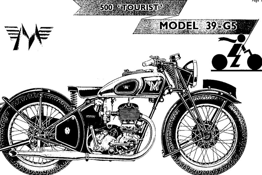
498 c.c. Side Valve, coil ignition
