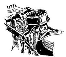
This neat and rigid speedometer mounting is a new feature for 1939 on most models. The dial is illuminated at night.
