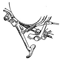
This single-arm side prop stand can be fitted to all 1939 models except the 39-G2 and 39-G7, at a small extra, and is strongly recommended to all MATCH-LESS owners.
